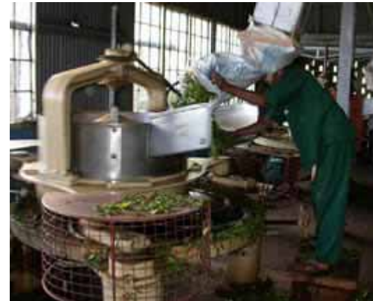
...into a grinding machine that pulverizes them and starts a fermentation process
