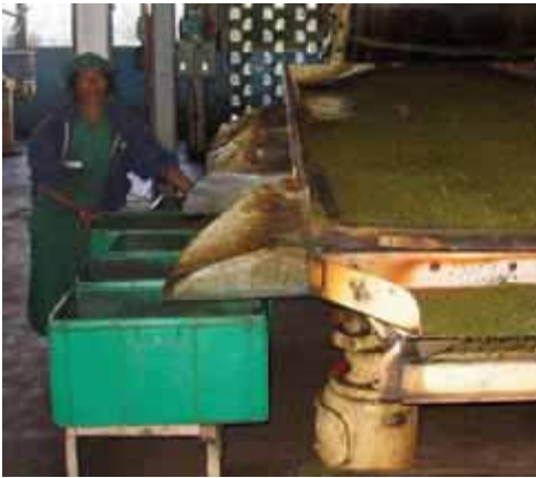
Freshly picked leaves are dehydrated by blowing air over them for 16 hours
